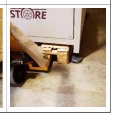
10. Put the fork lifter without the pallet under the machine and put it in the highest position possible 11. Screw in the feet until the lowest possible position
