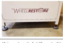
12. Lower down the fork lifter and pull it from underneath the machine to make the machine stands on its feet. Make sure all feet are in firm contact to the floor
