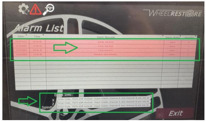
The identified error is displayed in the box below, accompanied by the following error code: 7829 eSM module: Input states channel A and channel B are not id.
