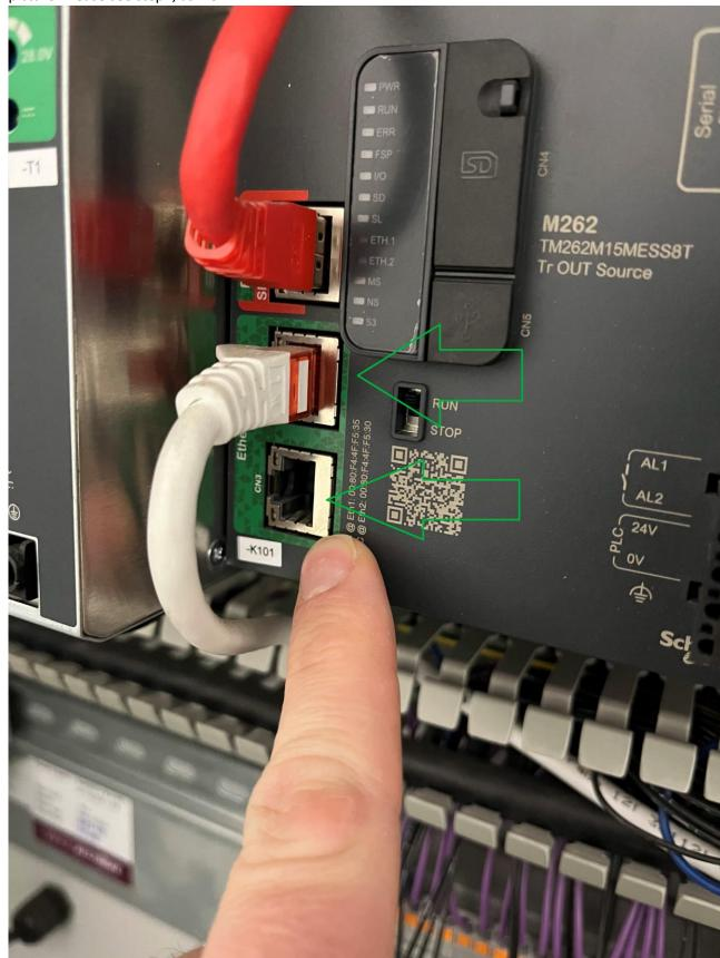
3. If that didn't work, try to switch the cable into the port below, that's marked as shown in the picture. Please see step4, as well.
