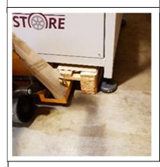
Remove the 4 feet from the machine and place them in the box inside the machine
