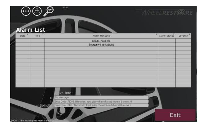
Most likely Cause: "Spinning" wheel or chuck/spindle manually too fast.
