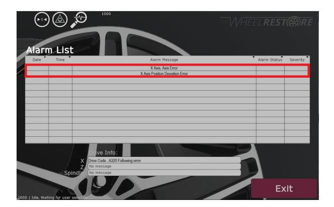
Most likely Cause: Limit switch on the left hand side of X axis is out of position.
