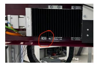
When.the.machine.is.homing?if.the.limit. switch.isn't.fully.covered.by.the.black.plate?the. alarm.will.be.triggered;.ln.the.image.below?you. can.see.the.limit.switch.is.not.fully.covered;
