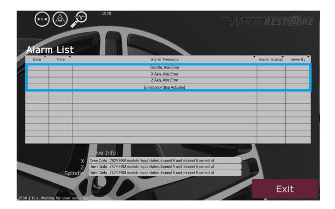
Most likely Cause: Foot pedal used incorrectly.
