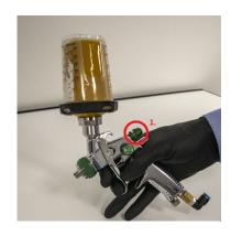
Opening of the trigger (#1.) of the paint gun is set to 3 MM.
