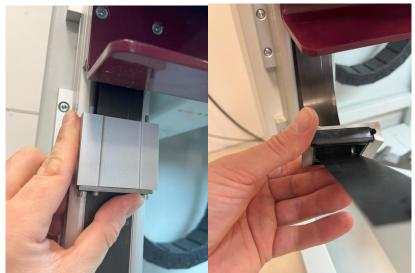
9. Now remove the top and lower black protection magnetic piece, and remove the little aluminimum, take the new black protection magnetic piece, and tape it together with the old one.
