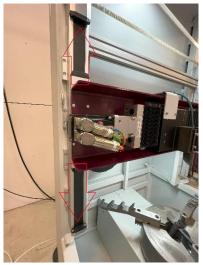
6. Then you need to use an Allen key, size 3 to remove the upper rubber part. You do the same for the lower bottom part.
