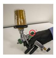
Opening of the trigger (#1.) of the paint gun is set to 3 MM.
