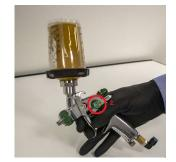
Operating pressure when using the paint gun is 2 bar
